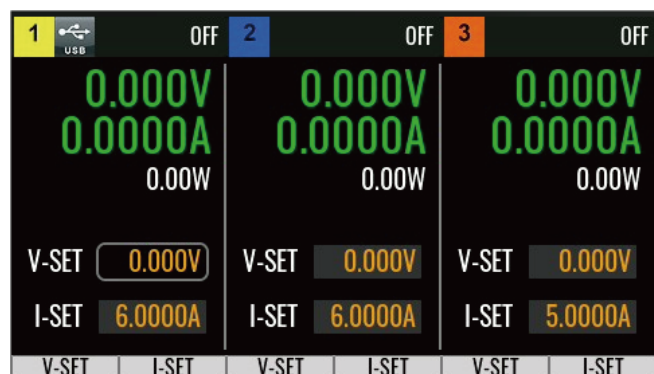
Triple-Channel Meter Interface and Quick Setup Interface
