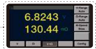
High speed simultaneous resistance and voltage measurement.
